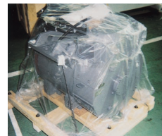
Reduced the amount of wood used in this simple fixed skid package.
