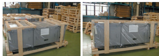
Simple packaging using wood beams. Structural innovations allow packaging with less wood than was used previously.
