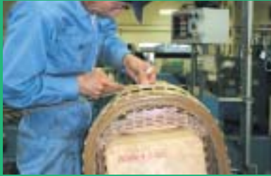
Coil winding process (displacement)
