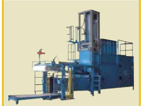
"Lacruz" Fully Automated "Other Plastic" Volume Reducing Packing Machine Engineered to reduce the volume of the waste category of "other plastic" unsuitable for recycling, to remove residue and other substances, and then to seal and package the plastic to create blast furnace recyclable materials. Nakayama Machinery Co., Ltd. Website: http://nakayamakikai.co.jp/ E-mail inquiries: info@nakayamakikai.co.jp
