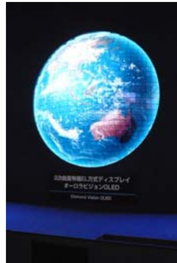
OLED display with semi-spherical surface
