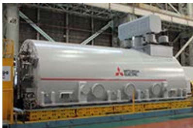
870MVA verified generator
