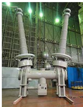
Gas circuit breaker
