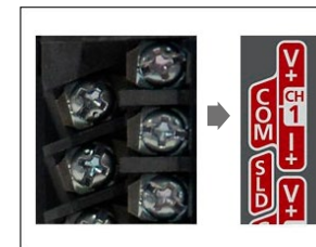
Print design illustrating the actual wiring
