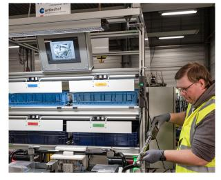
Thanks to the Poka Yoke controller, existing technology, like a digital torque wrench in this case, can easily be integrated into the error-free process with instructions fed to the operator via the GOT HMI.
