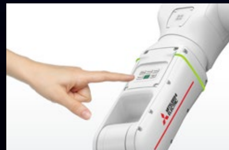
MELFA ASSISTA "Direct Teaching" instructions can be easily entered using the key pad at the top of the arm.
