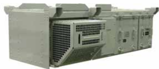
SiC auxiliary power supply systems for railcars
