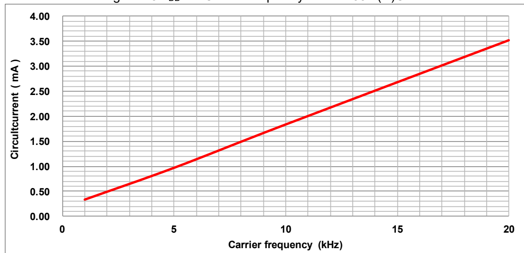
Fig. 4-2-6. I DB vs. Carrier frequency for PSS50M(N)C1F6
