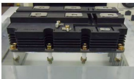
Fig.9-4 A HVIGBT module mounted on an acrylic plate
